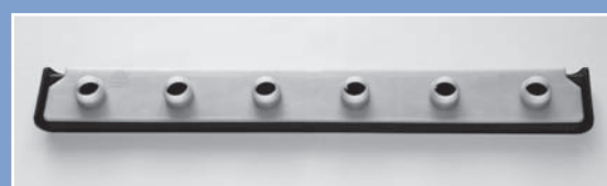
Lower part (black) made from PP regranulate, part weight 58.3 g + 1.5 g sprue, and cover, (white) made from PP+TPE, part weight 26.3 g + 1.5 g sprue; both produced in 4 cavities, with a cycle of between 24 and 30 seconds
