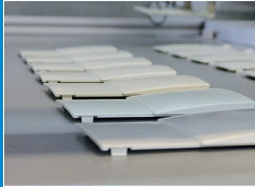
Both Venus II Machines with 1,500 kN clamping forces produce components for PLAYMOBIL® products
