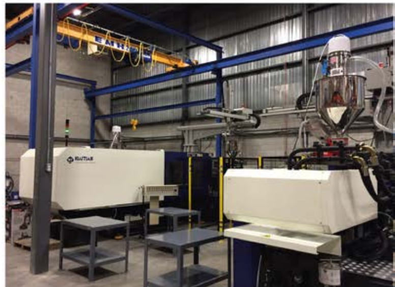
The new machine bay at DSI includes a Mars II 900 (101 U.S. tons), a Mars II 1200 (135 U.S. tons) and two Mars II 3200 (360 U.S. tons) machines. Absolute Haitian also arranged for automation on the the two larger machines.
