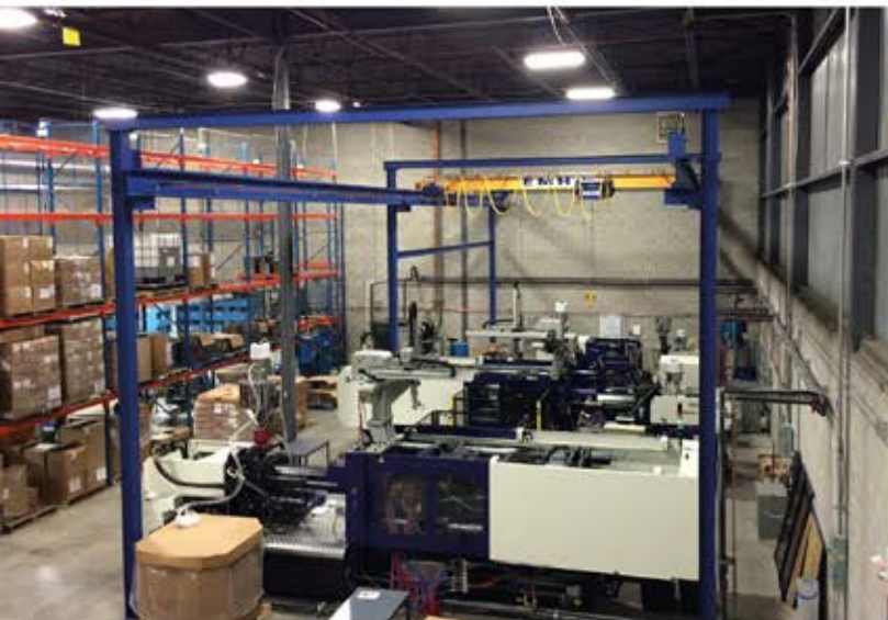
The new machine bay at DSI includes a Mars II 900 (101 U.S. tons), a Mars II 1200 (135 U.S. tons) and two Mars II 3200 (360 U.S. tons) machines. Absolute Haitian also arranged for automation on the the two larger machines.
