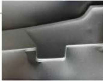
Car interior part made of PP with leather IMD with the Venus standard function "compression molding"
