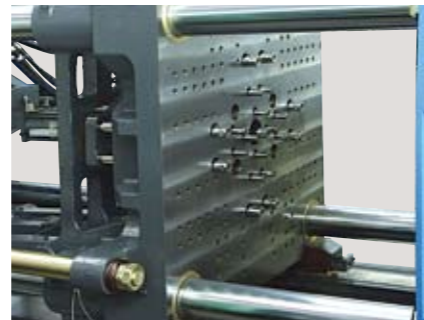
Euromap standard layout European standard layout of the platen ensure the flexibility of fixing mold.
