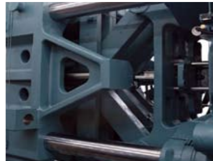
Dynamic and sensitive The 5-point double toggle provides short locking time and high opening forces.
